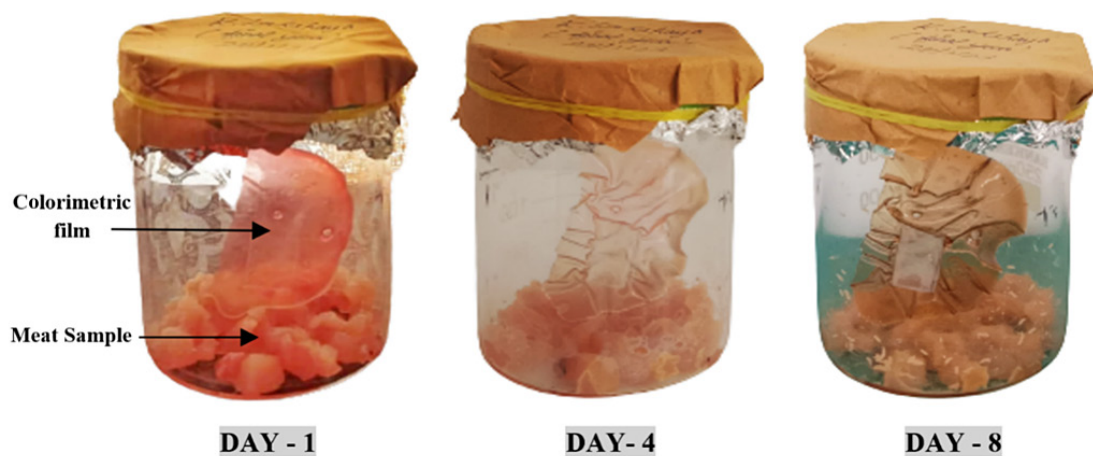
Fig. 11: Colorimetric film quality test on meat sample
